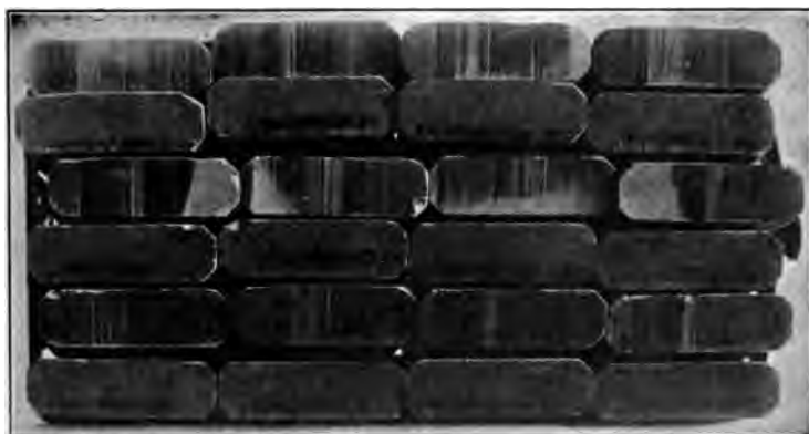
FIG. 83.—A full set of brushes placed on a machine without proper fitting. Note the small percentage of actual contact surface causing overloading and sparking.
